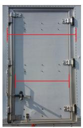
3/4" of clearance from edge of rivet to edge of rivet is required.
